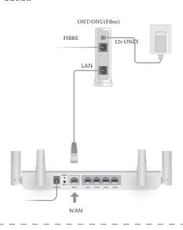
**3** Connect the router via **A** or **B** method.
