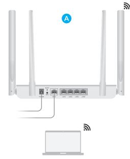
A Wi-Fi: Connect your device to the router's Wi-Fi using the SSID (network name) and Password printed on the bottom of the router.
